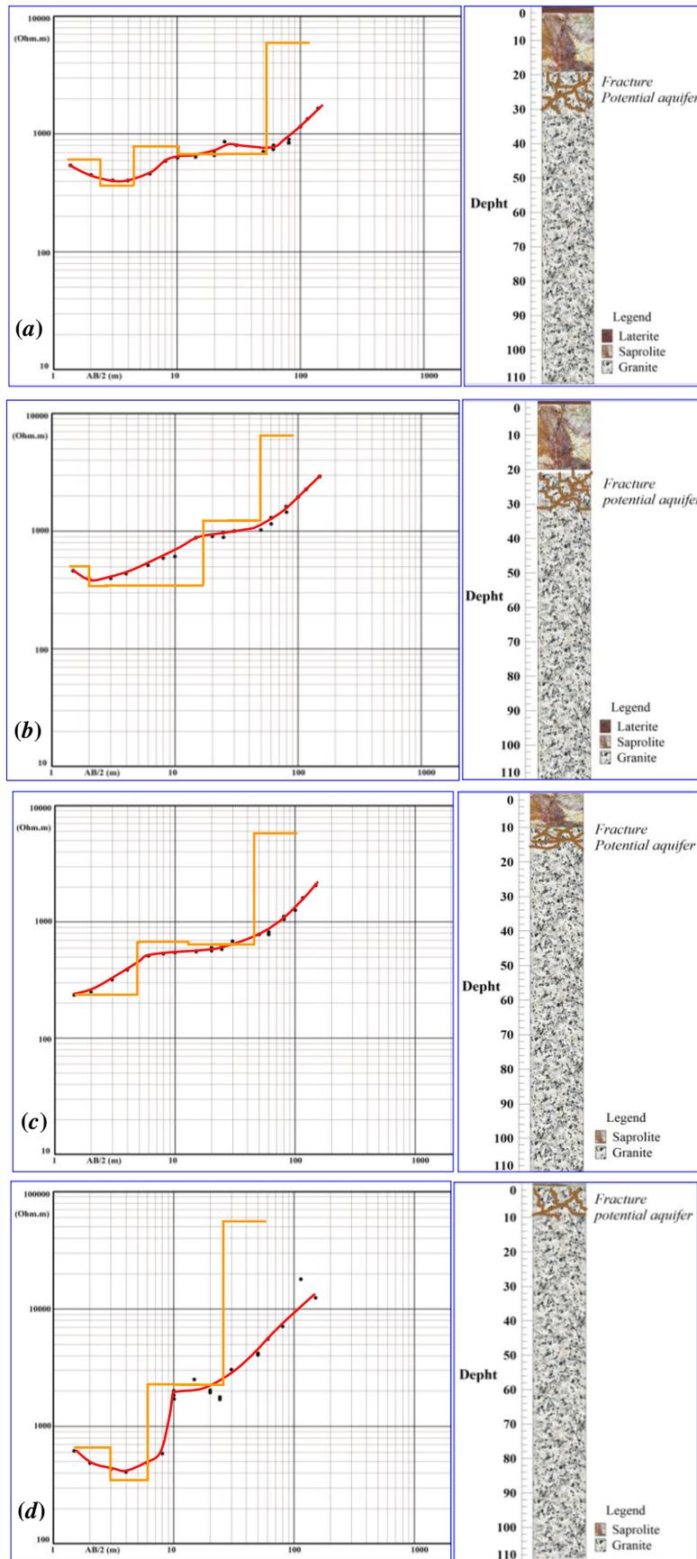
**Figure 5:** Electrical sounding curves and logs : (a) SD1/L150 N; (b) SD2/L300 N; (c) SD3/L500 N; (d) SD4/L700 N
