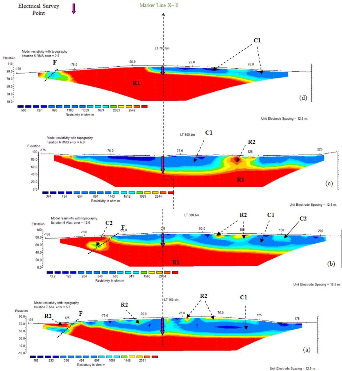
Figure 4: 2D section of selected profiles. (a) L150N, (b) L 300N, (c) L500N and (d) L 700N
