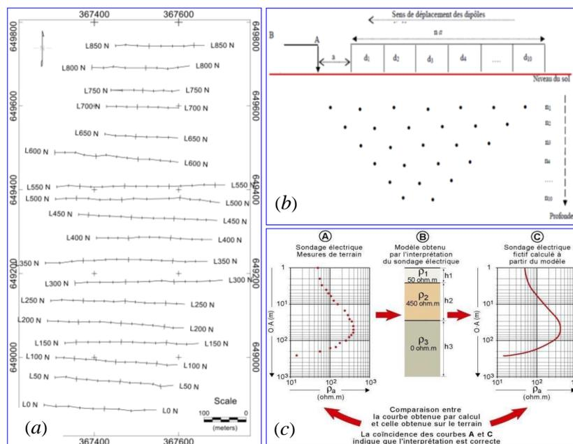
Figure 3: (a)-Profile positioning layout; (b)-Pôle-dipôle configuration; (c)- Technic of electrical survey curve inversion
